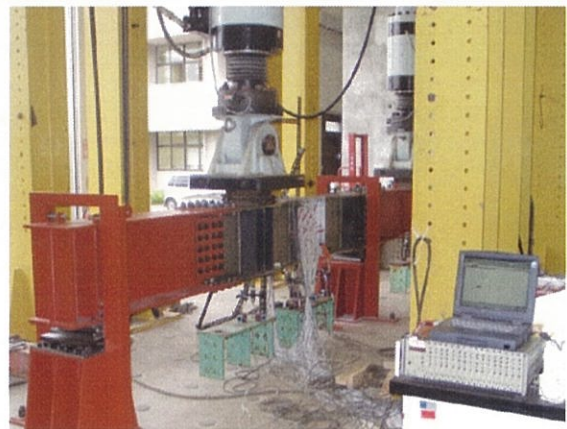
Ultimate shearing test of stainless steel plate girders
