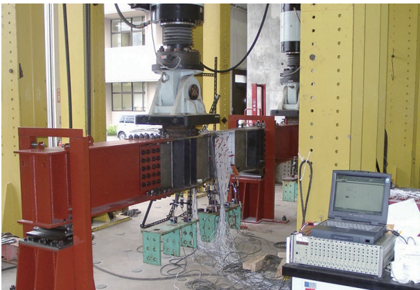
Ultimate shearing test of stainless steel plate girders
