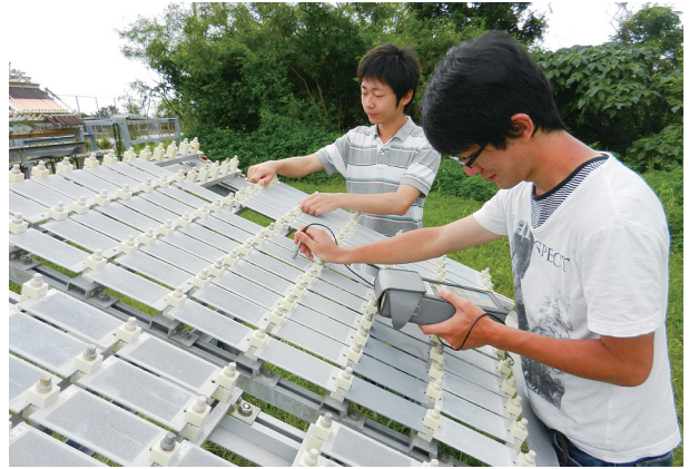
Atmospheric corrosion test for several metals
